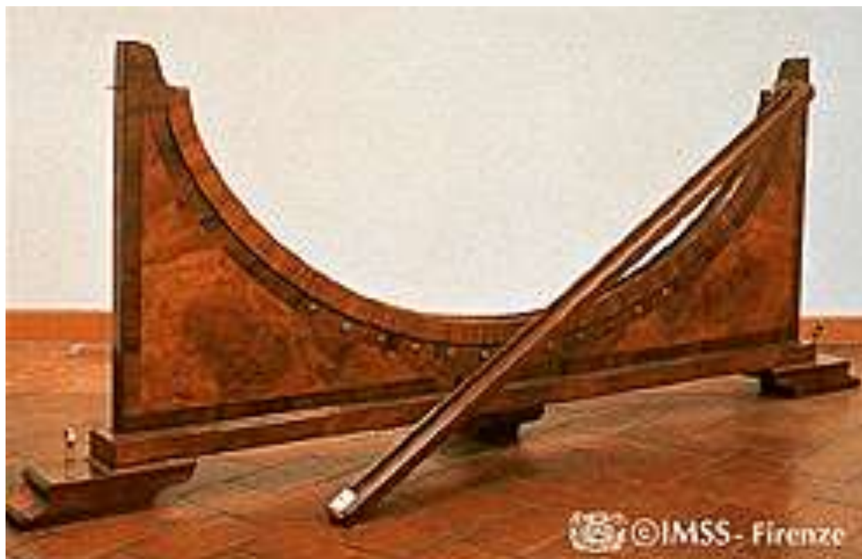
Figure 2 The cycloid curve or Brachistochrone curve is the curve of “shortest time” of descent under the condition of gravitation.
